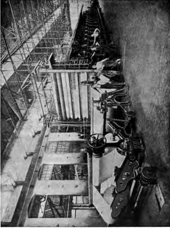
From the Twelfth United States Census. One of the largest paper machines in the world—162 inches wide.
